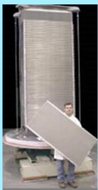
400-cell stack and individual cell package
